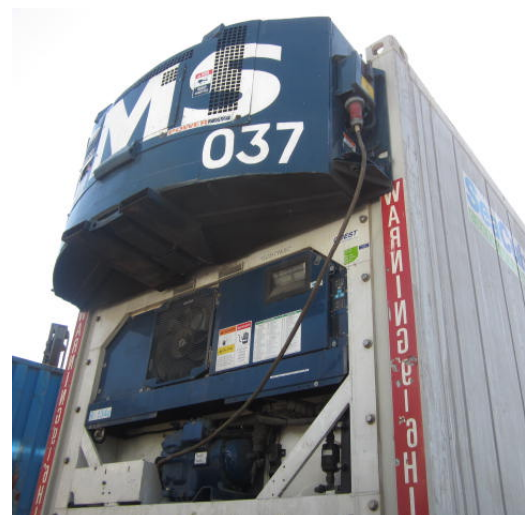
Photo: Reefer with extra backup genset
